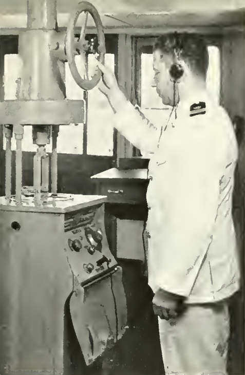
ONE OF THE FINEST SHIPBOARD RADIO INSTALLATIONS EVER CREATED WAS DESIGNED, BUILT, AND INSTALLED ON THE FORMER SS AMERICA BY RADIOMARINE CORPORATION OF AMERICA. LEFT: RADIO DIRECTION FINDER IN THE "WHEEL HOUSE." ABOVE: THE SHIP'S MAIN RADIO OPERATIONS ROOM.
