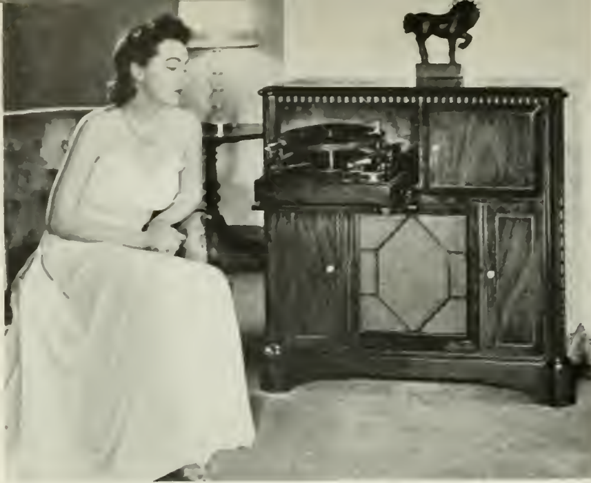
BEFORE THE WAR TERMINATED DOMESTIC MANUFACTURING ACTIVITIES, A HIGH MARK IN CRAFTSMANSHIP WAS REACHED IN THIS RCA 10-TUBE COMBINATION RADIO-PHONOGRAPH INSTRUMENT.
